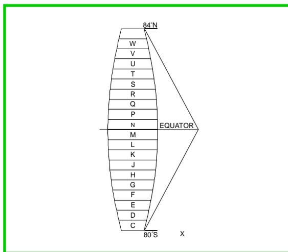
Figure 1.4.3: Grid Segments of the UTM Grid System.
