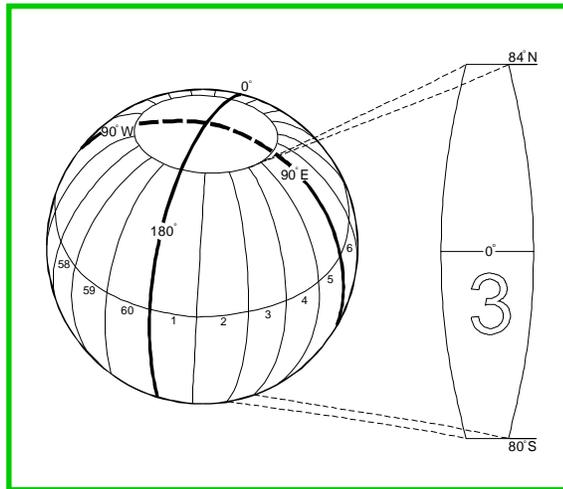
Figure 1.4.2: Grid Zones of the UTM Grid System.
