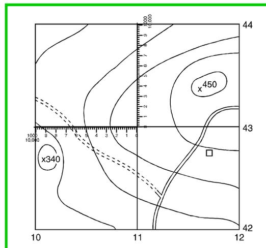
Place the horizontal scale parallel to and directly on top of grid line 43 with the "0 mark" at the lower left corner of grid square YF1143 (see Figure 1.4.9).
