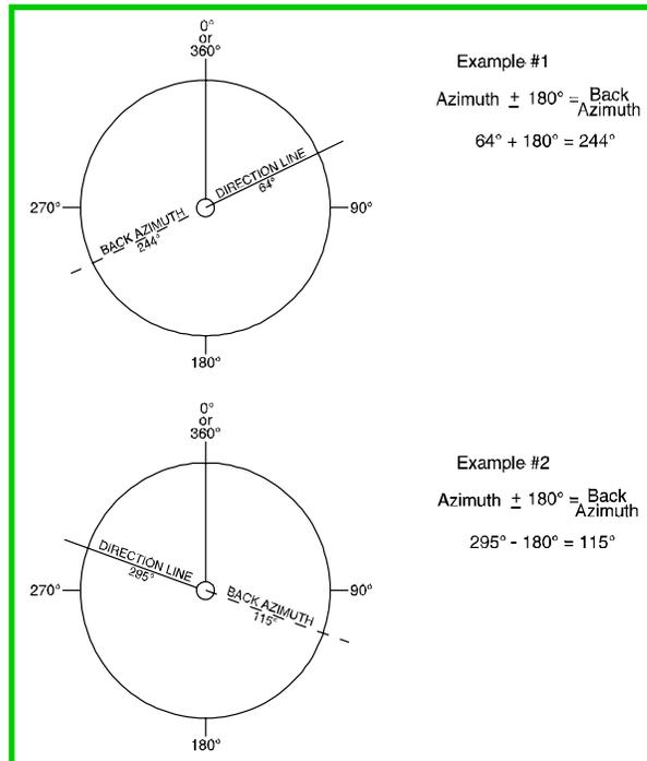
A magnetic azimuth is a direction expressed as the angular difference between magnetic north and the direction line (see Figure 1.7.4). You can determine a magnetic azimuth using a compass or other magnetic instrument (such as surveying equipment).
