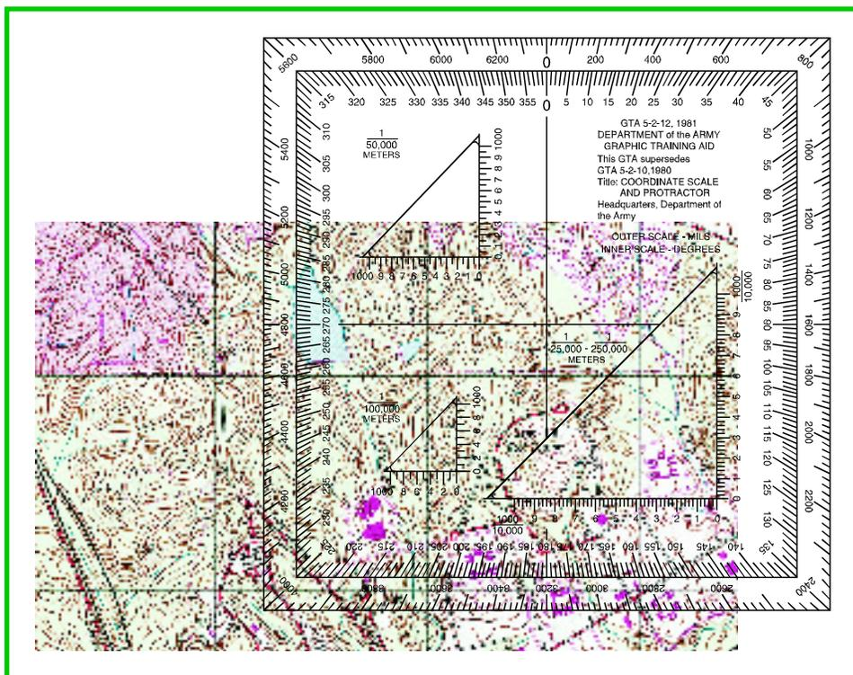
Figure 1.7.10: Using a protractor to plot a grid azimuth.
