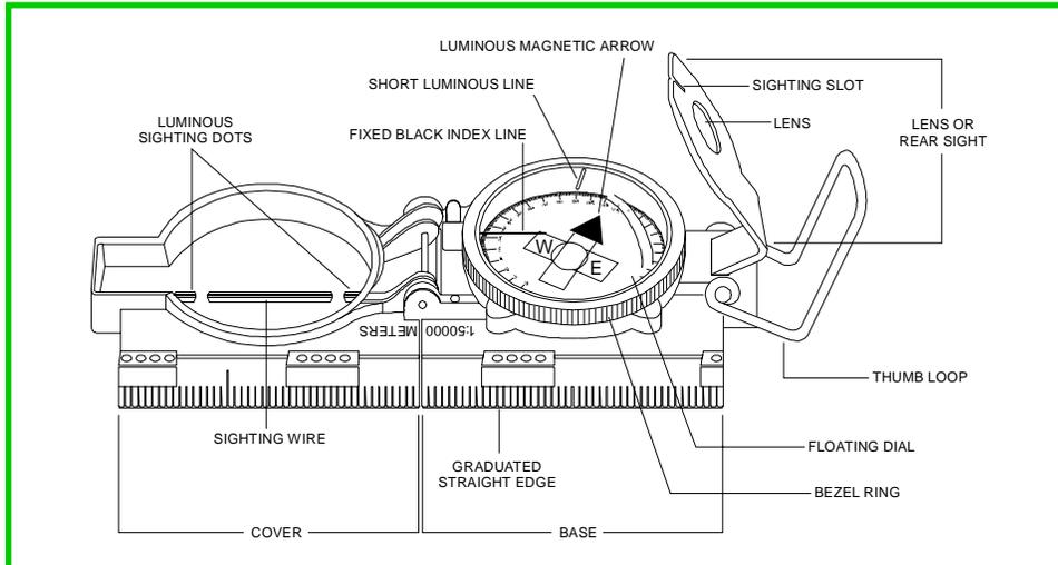
Figure 1.7.5: The magnetic lensatic compass.
