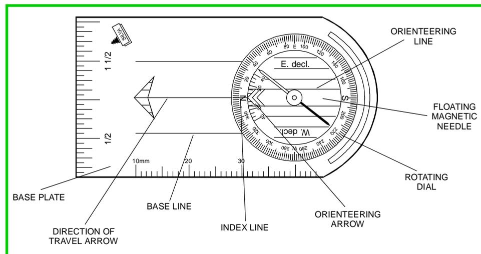
The floating needle is mounted on a pivot so that it can rotate freely when you hold the compass level. It settles within four seconds, always pointing to magnetic north. Printed distinctly on the rotating dial are the letters N and S, to represent 0/360 degrees and 180 degrees, respectively. The dial is graduated at two degree intervals, marked at 20 degree intervals, and contains the letters E (at 90 degrees) and W (at 270 degrees).
