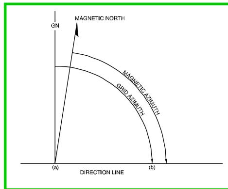
Figure 1.7.4: Magnetic and grid azimuths.
